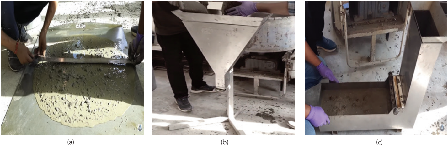
Figure 7: Experimental setup for (a) Slump flow, (b) V-funnel, and (c) L-Box test
