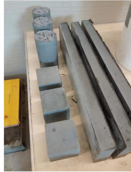
Figure 6: Some typical specimens after demoulding
