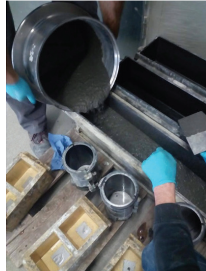
Figure 4: Casting of specimens
