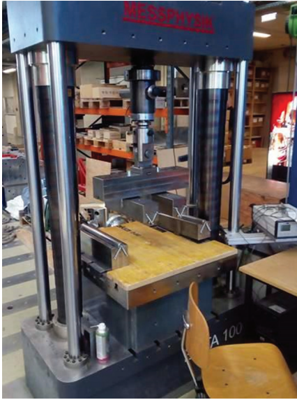
Figure 5: Test setup for four-point bending tests
